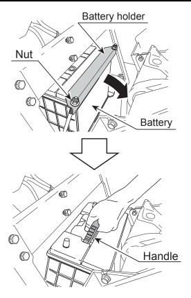
Figure 35. Removing Battery
